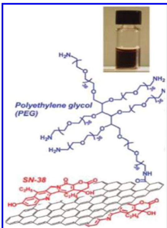
Figure 17. Immobilization of SN38 camptothecin on PEG-GO. Reprinted with permission from ref 110. Copyright 2008 American Chemical Society.
