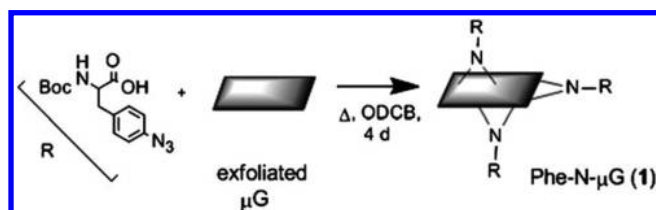
Figure 8. Nitrene addition to graphene sheets using Boc-protected azidophenylalanine. Reprinted with permission from ref 84. Copyright 2010 Royal Society of Chemistry.
